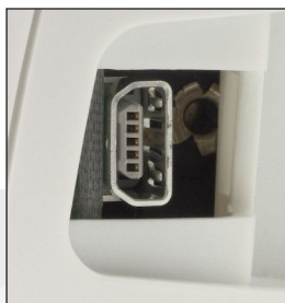
Above: Detail of USB socket
